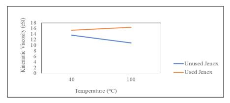
Figure 2 Viscosity against temperature of Jenox brake fluid
