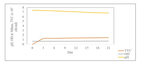
Figure 3 Growth profile of A. flavus in unused Abro brake fluid
