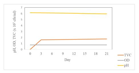
Figure 7 Growth profile of A. flavus in used Jenox brake fluid
