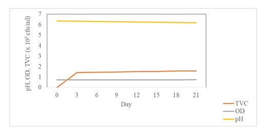
Figure 6 Growth profile of A. flavus in unused Jenox brake fluid
