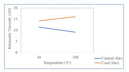
Figure 1 Viscosity against temperature of Abro brake fluid
