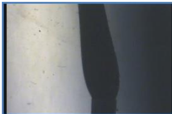
Figure 12 Flowing stream of oil resulting from ultra-low IFT
