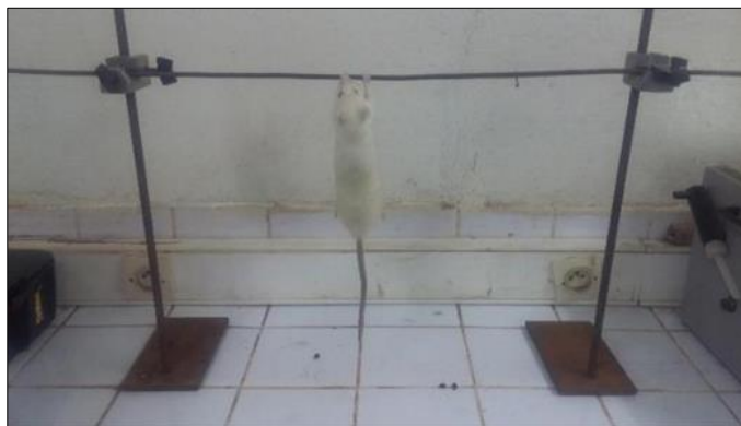
Figure 4 Grip test device (photographed by TCHIESSO on 18/11/2015)
