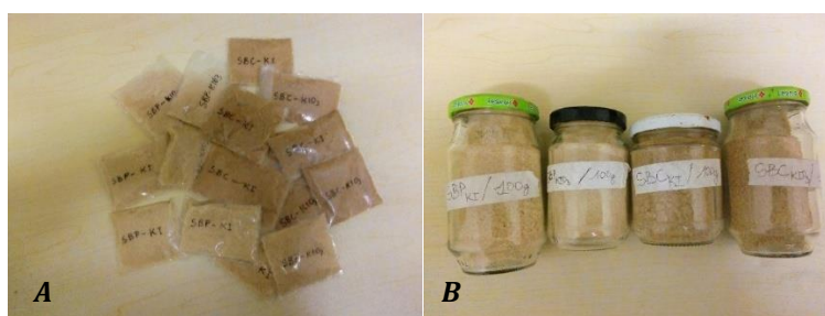
Figure 4 Plant salts packaged in: A- high density polyethylene (HDPE) bags; B- glass jars
