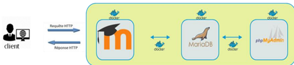
Figure 2 Web server architecture based on docker
