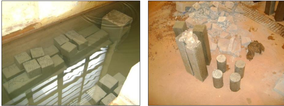
Figure 3 (a) Test Samples in the curing Tank (b) Some of the Test Samples after removal from the curing Tank
