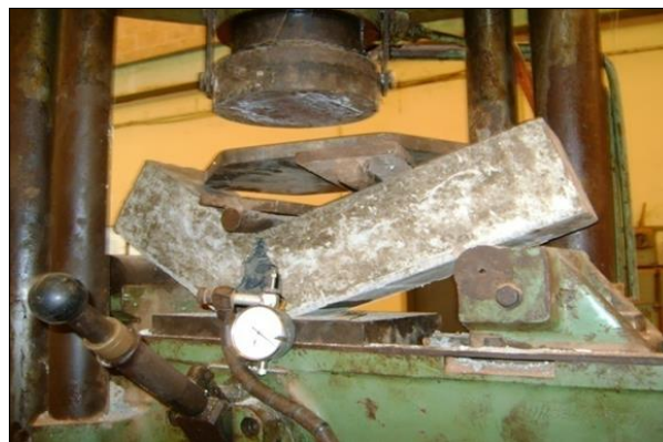
Figure 4 A failed beam tested for the determination of the modulus of Rupture
