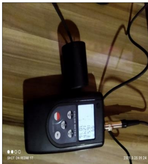
Figure 1 Lander Color meter, model: CM200S with serial number N974978
