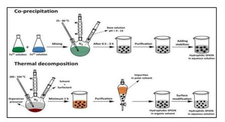
Figure 14 Synthesis of iron oxide by co-precipitation and thermal decomposition method [168]
