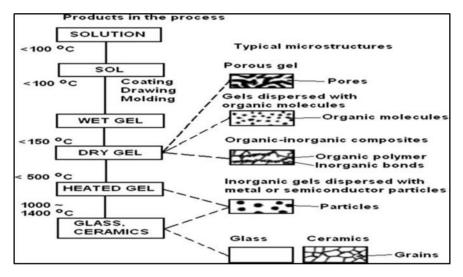
Figure 16 Flow diagram for the development of different types of nanoparticles [185]
