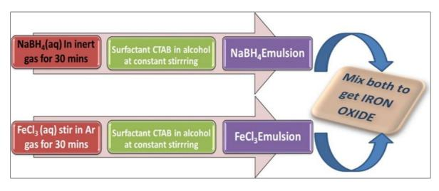
Figure 15 Mechanism for the formation of iron oxide nanoparticles by micro-emulsion method [170]
