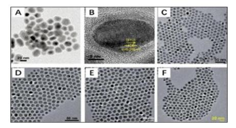
**Figure 10** (A and B) TEM AND HRTEM images of iron carbide and crystalline morphology of iron carbide in (C,D,E,F) as hexagonal and monoclinic Fe<sub>2</sub>C, monoclinic Fe<sub>5</sub>C<sub>2</sub> and orthorhombic Fe<sub>3</sub>C respectively [80,81]
