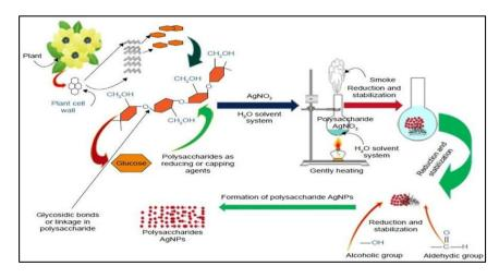
Figure 20 Schematic diagram for the development of Ag nanoparticles via green synthesis [194]
