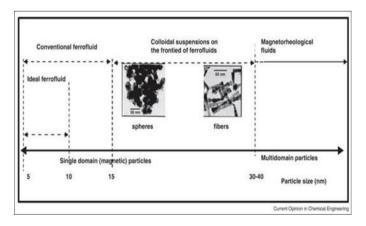
Figure 8 Classification of magnetic ferrofluids [74]
