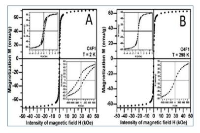
Figure 7 A and B Magnetic properties or chitosan coated magnetite at 2K and 298 K respectively [77]
