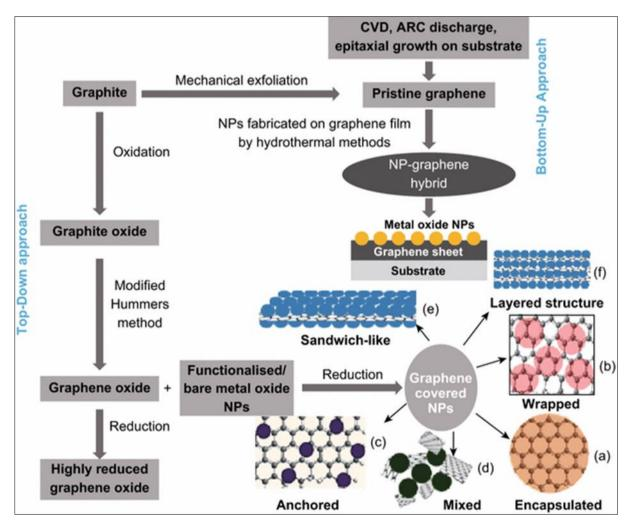
Figure 12 Flow chart with graphene synthetic routes for graphene and different types of graphene nano hybrids [90]
