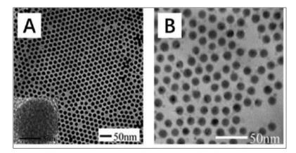
Figure 5 TEM images of Fe-Pd alloy (AandB) with particle size 11 and 16nm respectively. [68]
