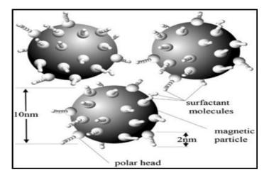
Figure 6 Surface functionalization of MNPs in ferrorfluids. [73]
