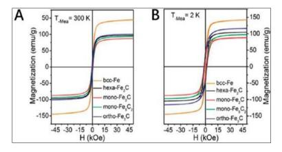
Figure 9 Ferromagnetic behavior of iron carbide at different temperatures A 300K and B 2K [81]
