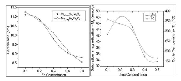
Figure 3 and 4 Reduction of Particle size by incorporation of Zn particles at room temperature and Effect of Zn doping on specific magnetization and Curie temperature [42]
