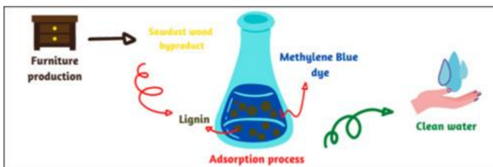
Figure 7 Animated scheme shows the adsorption process of methylene dye on the extracted lignin surface [43]
