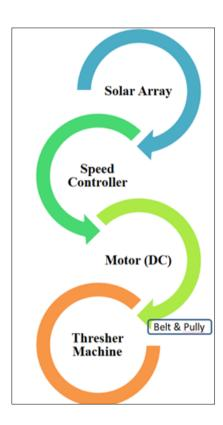
Figure 1 Power transmission system of developed paddy thresher for operation
