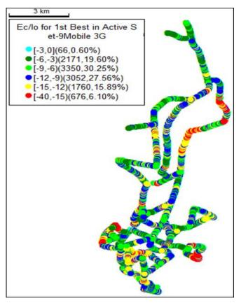
Figure 5 UMTS Quality Plots for 9mobile Mobile Network
