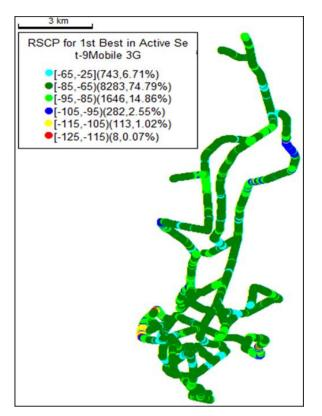
Figure 1 UMTS Coverage Plots for 9mobile Mobile Network
