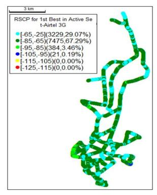
Figure 4 UMTS Coverage Plots for Airtel Mobile Network
