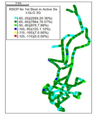
Figure 2 UMTS Coverage Plots for Globacom Mobile Network
