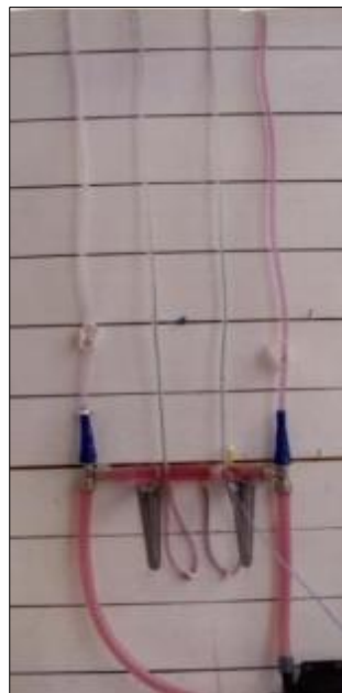
Figure 15 The G tube in G-C apparatus connected to circulatory model driven by electric pump. The proximal pressure (PP) akin to arterial pressure is above 100 cm water when the distal pressure (DP) is less than 7 cm water (hidden behind the blue tube). The pressure in the chamber around the G tube is less than DP. Furthermore, the pressure in C manometers is lower near the inlet than it is near the exit. So, suction or reabsorption of fluid occurs through side holes
