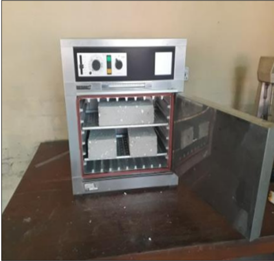
Figure 3 Blocks are dried in an oven.
