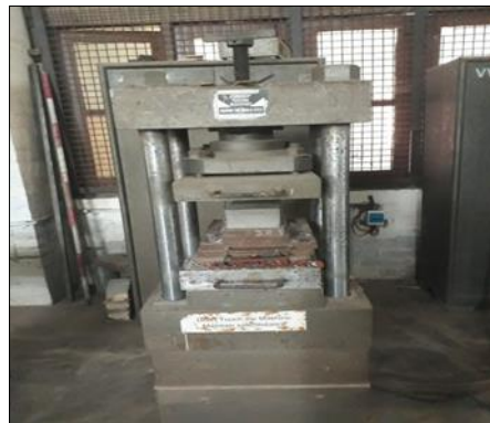
Figure 5 Compressive strength test of blocks
