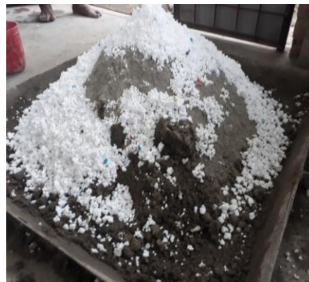
Figure 2 Mixing cement–sand–expanded polystyrene
