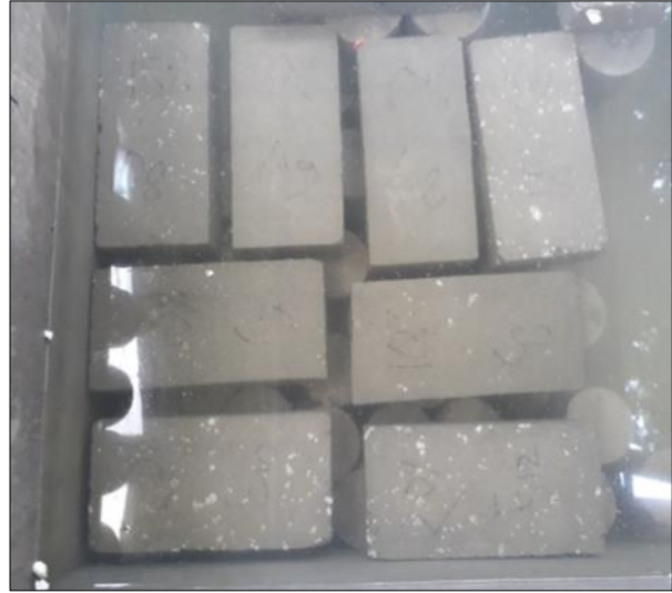
Figure 4 Blocks are immersed in water
