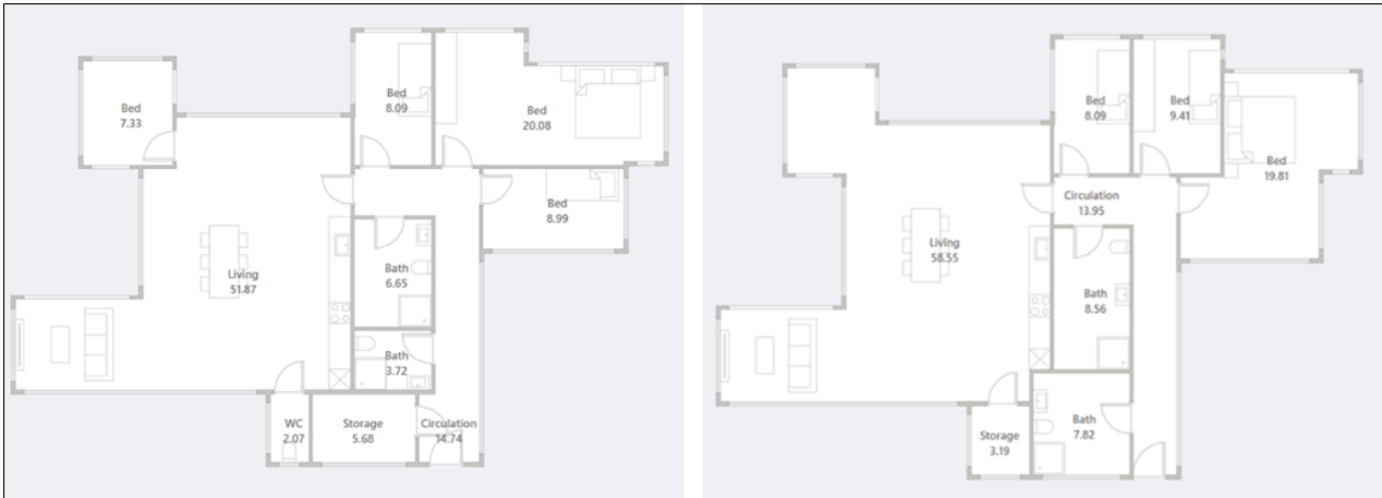
Figure 3 Plans generated by PlanFinder based on initial input specifications (14).
