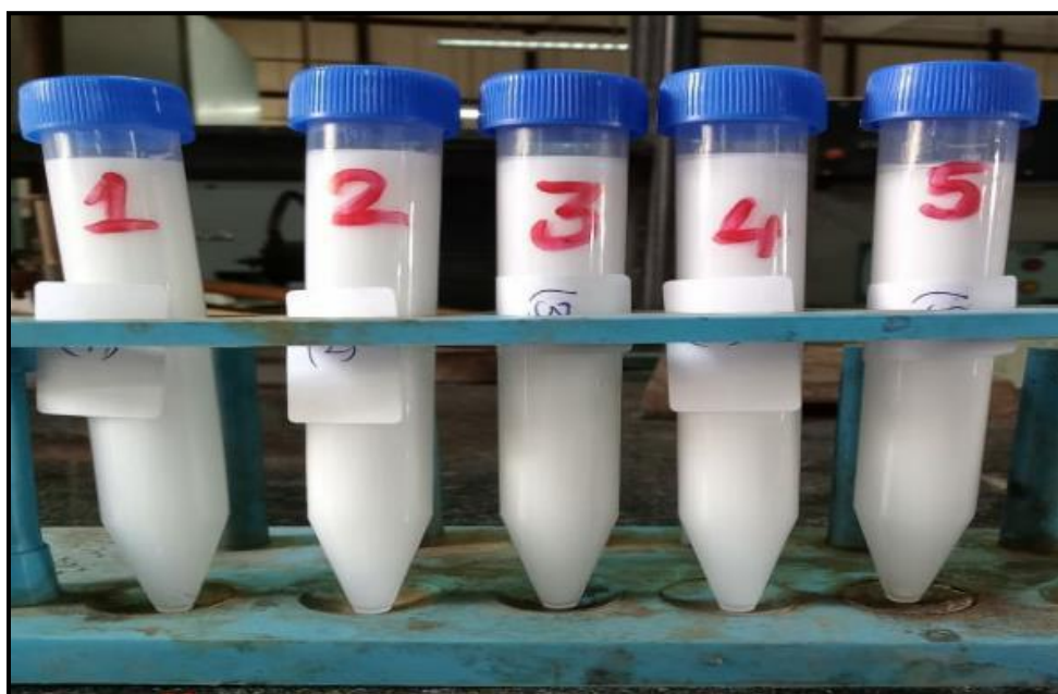
Figure 5 Set of Pickering Emulsion with water, Eucalyptus Oil and nanocellulose
