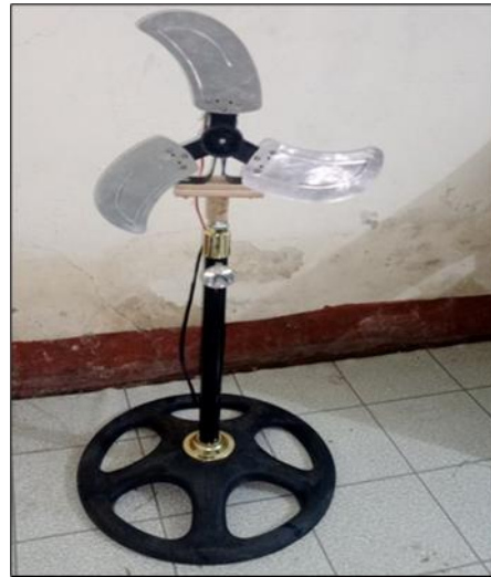
Figure 9 The completed assembly of the mini wind turbine
