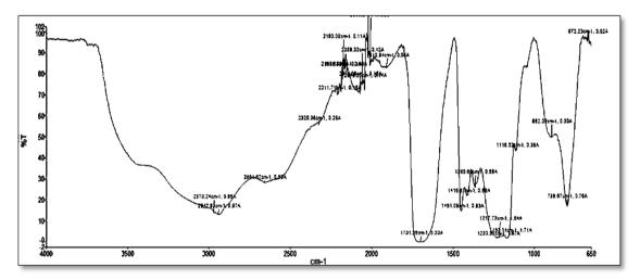
Figure 2 FTIR spectra of carbomer 940
