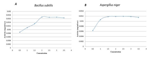
Figure 3 Optimization of substrate concentrations for cellulase production by microbial isolate form cassava waste water
