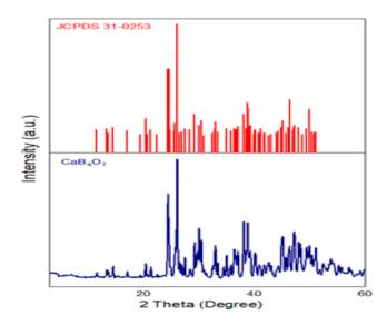
Figure 1 The X-ray pattern of synthesized calcium tetraborate
