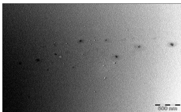
Figure 6 TEM image of synthesized CuONPs
