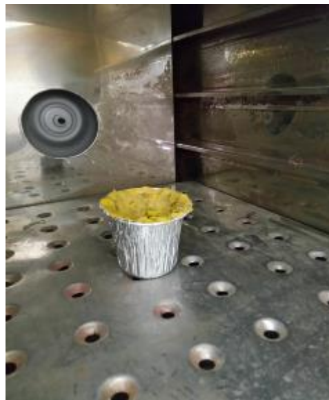
Figure 8 Mixture was baked in oven at 130°C for one hour by using a mold
