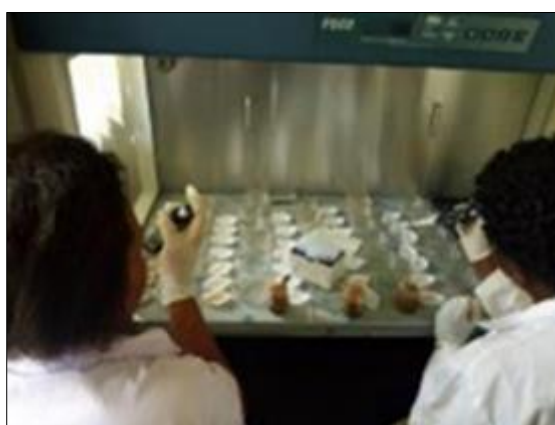
Figure 2 Research team performing serial dilutions of soil under laminar flow prior to culturing on PDA and SDA (fungi) and MRS agar (bacteria) (Photo credit: Ronald Kisekka)
