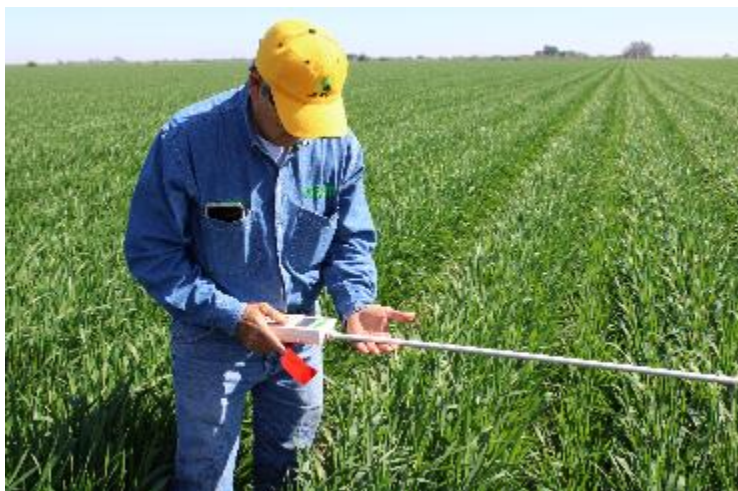
Figure 2 Taking readings of the leaf area index using a linear ceptometer AccuPAR LP-80.
