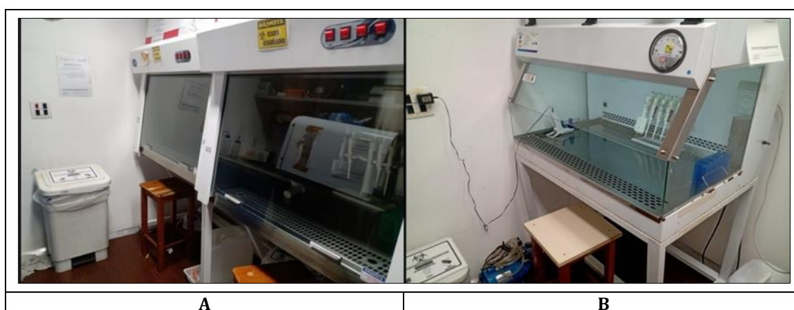
Figure 1 (A) model with a UV filter on the glass. (B) model without UV filter.
