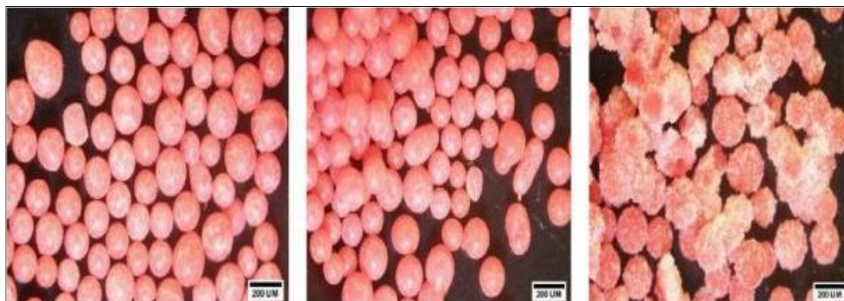
Figure 3 Microbeads of product (A16) heated at 60^\circ\text{C} , 80^\circ\text{C} and 100^\circ\text{C}
