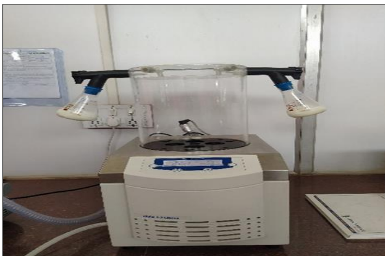
Figure 4 Manifold method of Lyophilization
