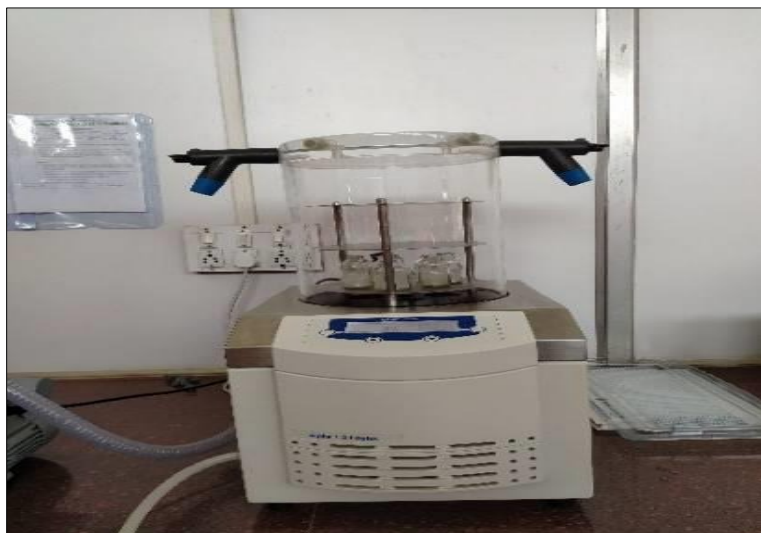
Figure 5 Batch method of Lyophilization
