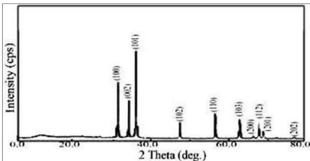
**Figure 2** XRD graph of ZnO nanoparticles
