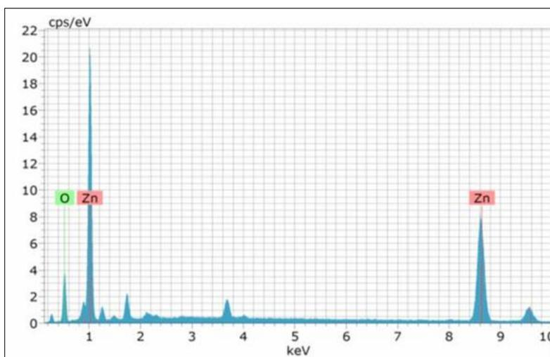
**Figure 4** EDAX image of ZnO nanoparticles
