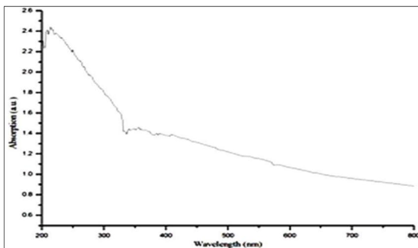
**Figure 6** UV-Visible spectroscopy graph of ZnO nanoparticles
