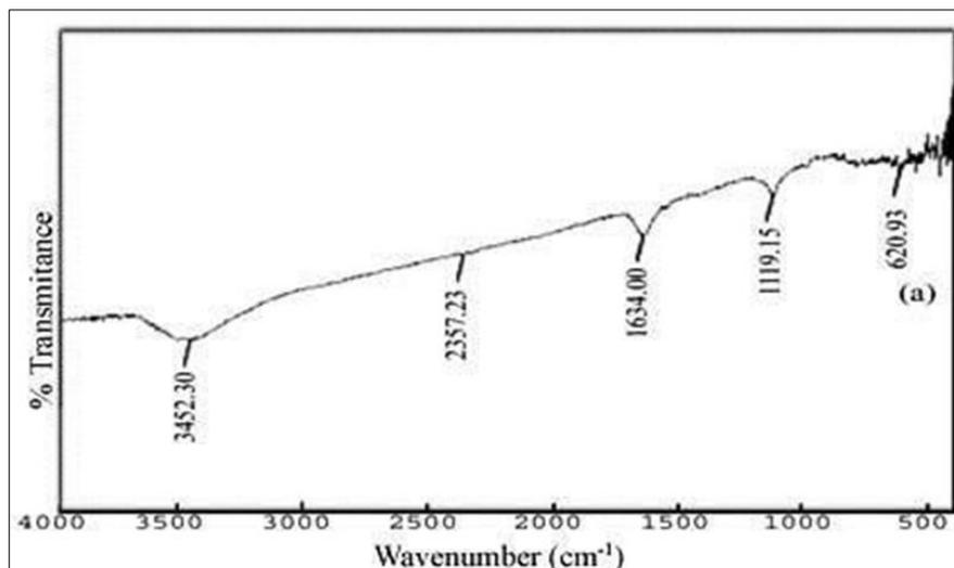
**Figure 5** FTIR spectrum of ZnO nanoparticles
