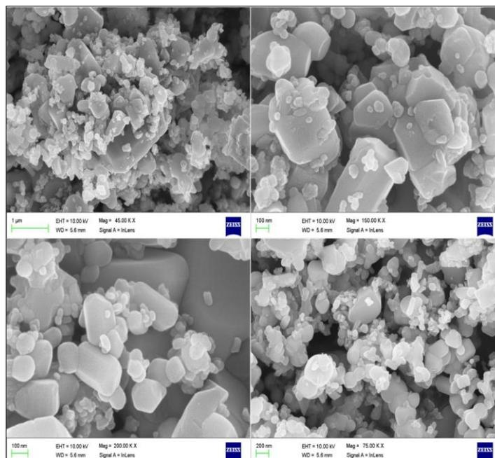
**Figure 3** SEM image of ZnO nanoparticles
