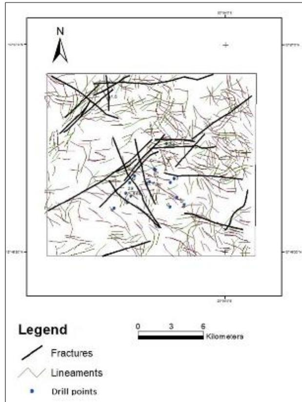
**Figure 10** Drilling data overlaid on the fracturing map
