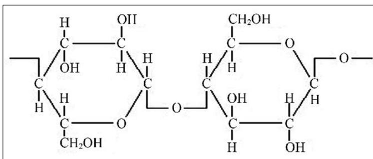
**Figure 7** Structure of Cellulose
