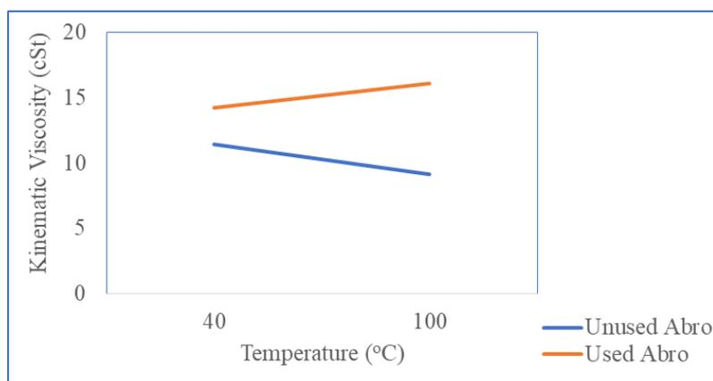
**Figure 1** Viscosity against temperature of Abro brake fluid
