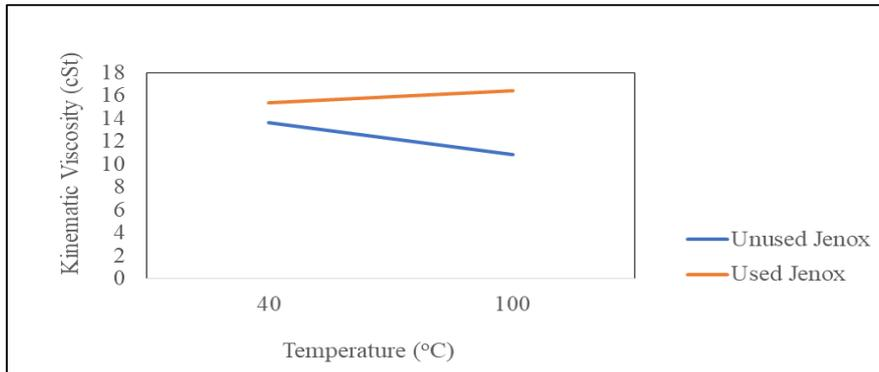
**Figure 2** Viscosity against temperature of Jenox brake fluid
