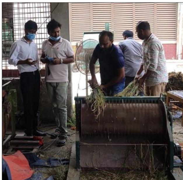
**Figure 2** Thresher performance test
