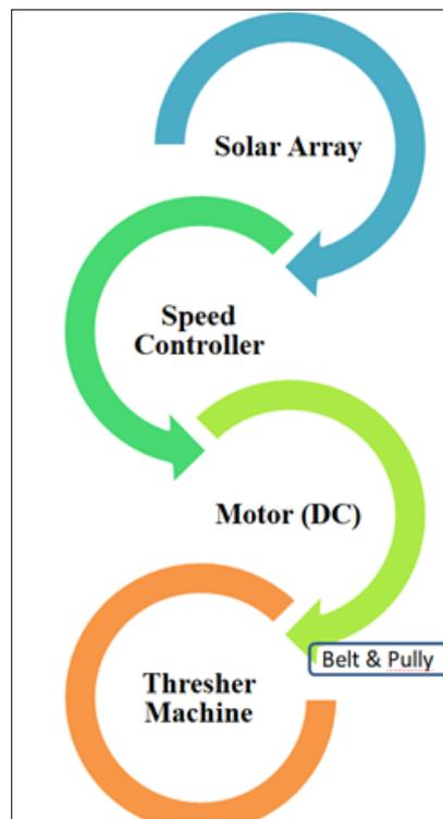
**Figure 1** Power transmission system of developed paddy thresher for operation
