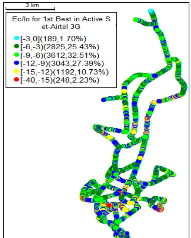
Figure 8 UMTS Quality Plots for Airtel Mobile Network
