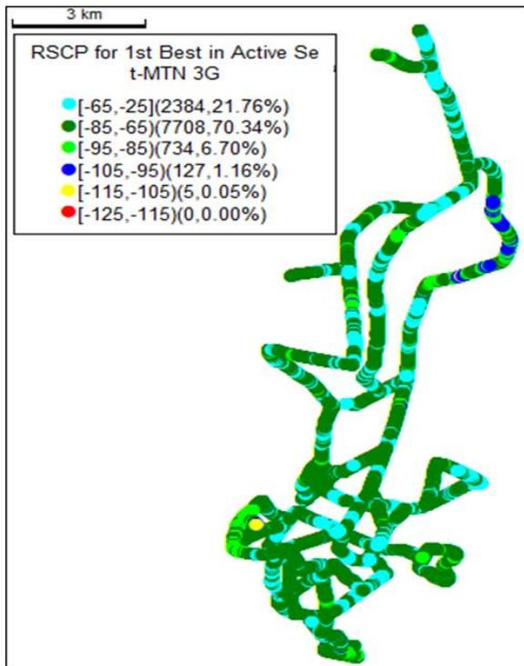
**Figure 3** UMTS Coverage Plots for MTN Mobile Network
