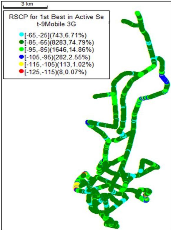
**Figure 1** UMTS Coverage Plots for 9mobile Mobile Network
