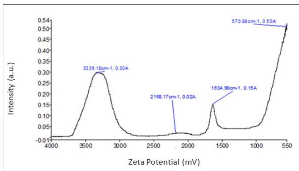
**Figure 3** FTIR graph showing the functional groups predicted in silver nanoparticle
