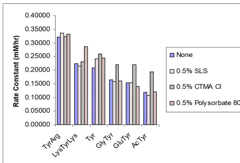
**Figure 1** Effect of different surfactants on the rate of photo-degradation of model tyrosyl compounds (2mM) at pH 10 (simulated solar irradiance = 760 W/m<sup>2</sup>)
