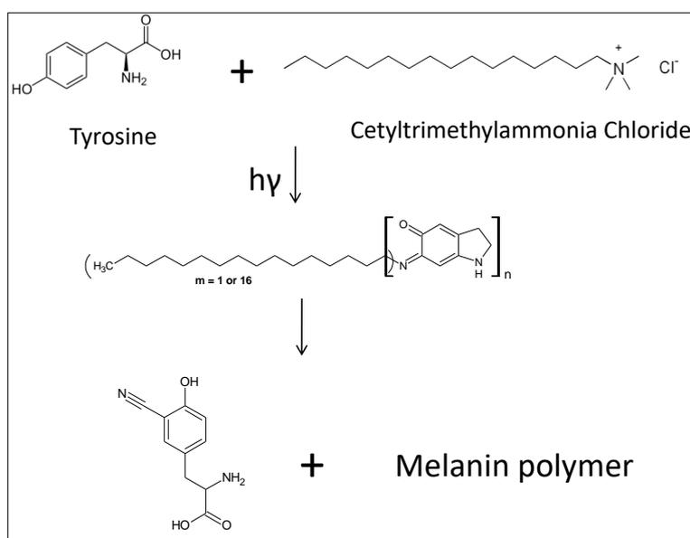
**Figure 2** Formula of photochemical reaction between tyrosine and Cetrimonium chloride
